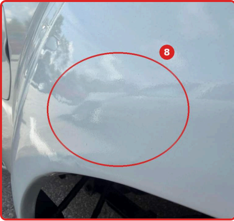
#8 Driver-side bed panel: waviness consistent with prior repair and repaint
