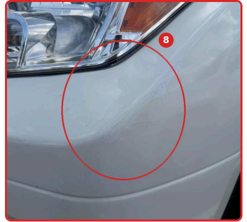
#8 Front bumper corner: scuffing with brush touch-up paint
