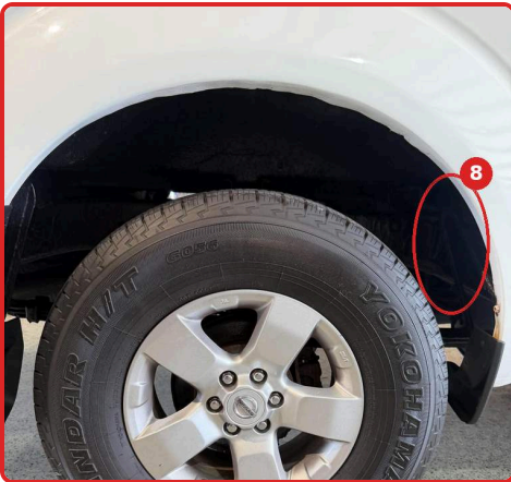
#8 Rear wheel arch lip: rust bubbling at the edge
