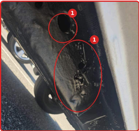
#1 Frame rail: pitted, perforated metal sprayed over with fresh black undercoating
