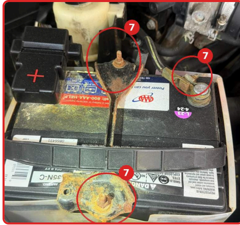
#7 Battery hold-down heavily rusted; negative terminal corroded
