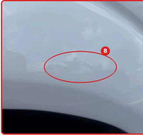
#8 Bed panel: paint texture change indicating refinish
