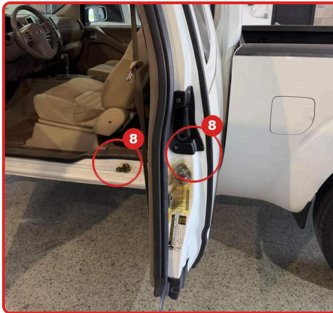
#8 Door sill and B-pillar: rust at fastener points
