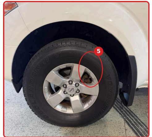
#5 Front caliper seen through the wheel: heavy rust
