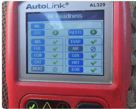
Scan: MIL off, 0 codes, monitors complete
