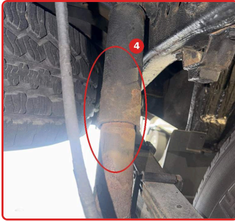
#4 Rear shock absorber: heavily corroded body
