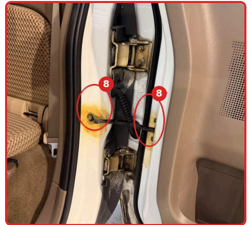
#8 Rear door hinge area: rust bleeding at the mounts
