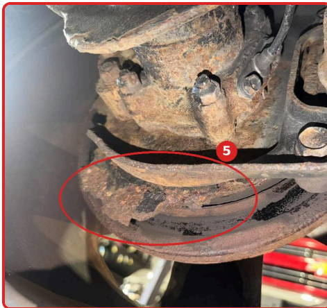
#5 Front dust shield rusted through and separating; rotor edge rusted
