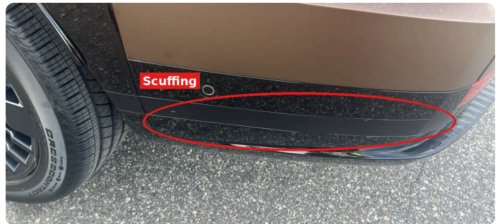
Rear bumper lower strip: scuffing
