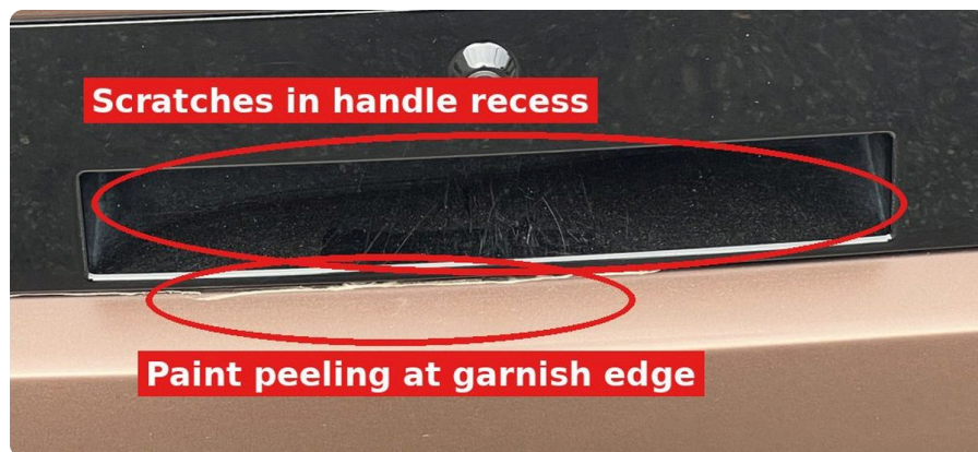
Liftgate garnish: paint peeling along the bottom edge and scratches inside the handle recess
