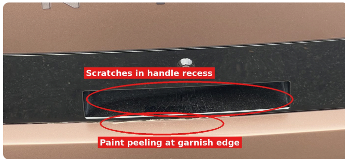
Liftgate: paint peeling at the garnish edge, scratches in the handle recess
