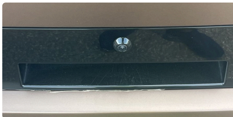
Liftgate garnish, second angle: scratches across the handle recess and peeling at the lower edge
