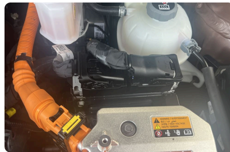
Coolant reservoirs and HV components
