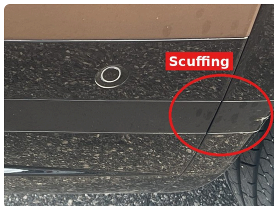
Rear bumper corner: scuffing on the lower gloss black and matte strips near the tire
