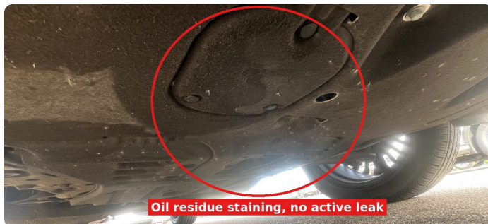
Underbody shield: oil residue staining, no active leak
