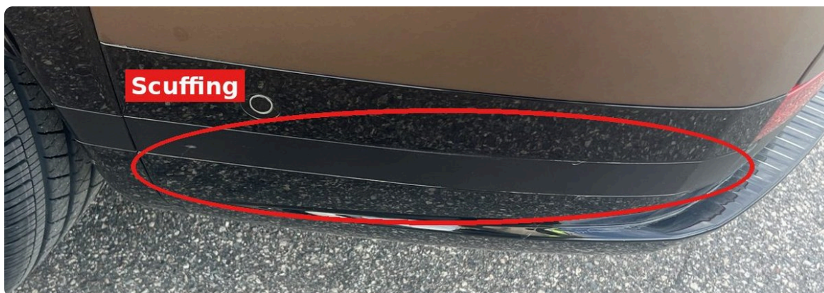
Rear bumper lower strip, opposite corner: scuffing along the matte strip
