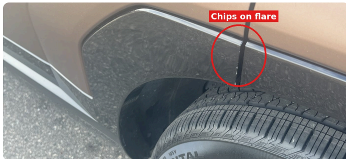
Rear wheel arch flare: chips
